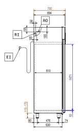
Electrical inlet (power) Refriaerant Inlet Refrigerant Outlet
